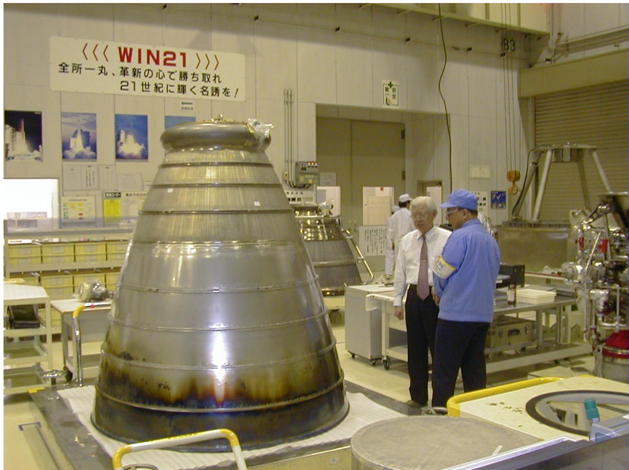
No. 8-2: The nozzle skirt of the LE-5B engine
