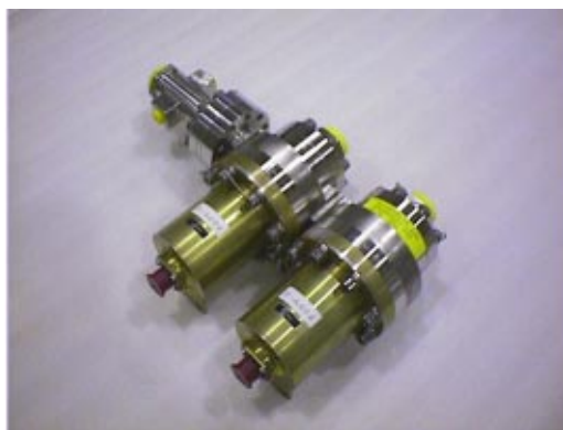
(No. 7: 2 stages liquid oxygen tank pressure adjustment valve)
