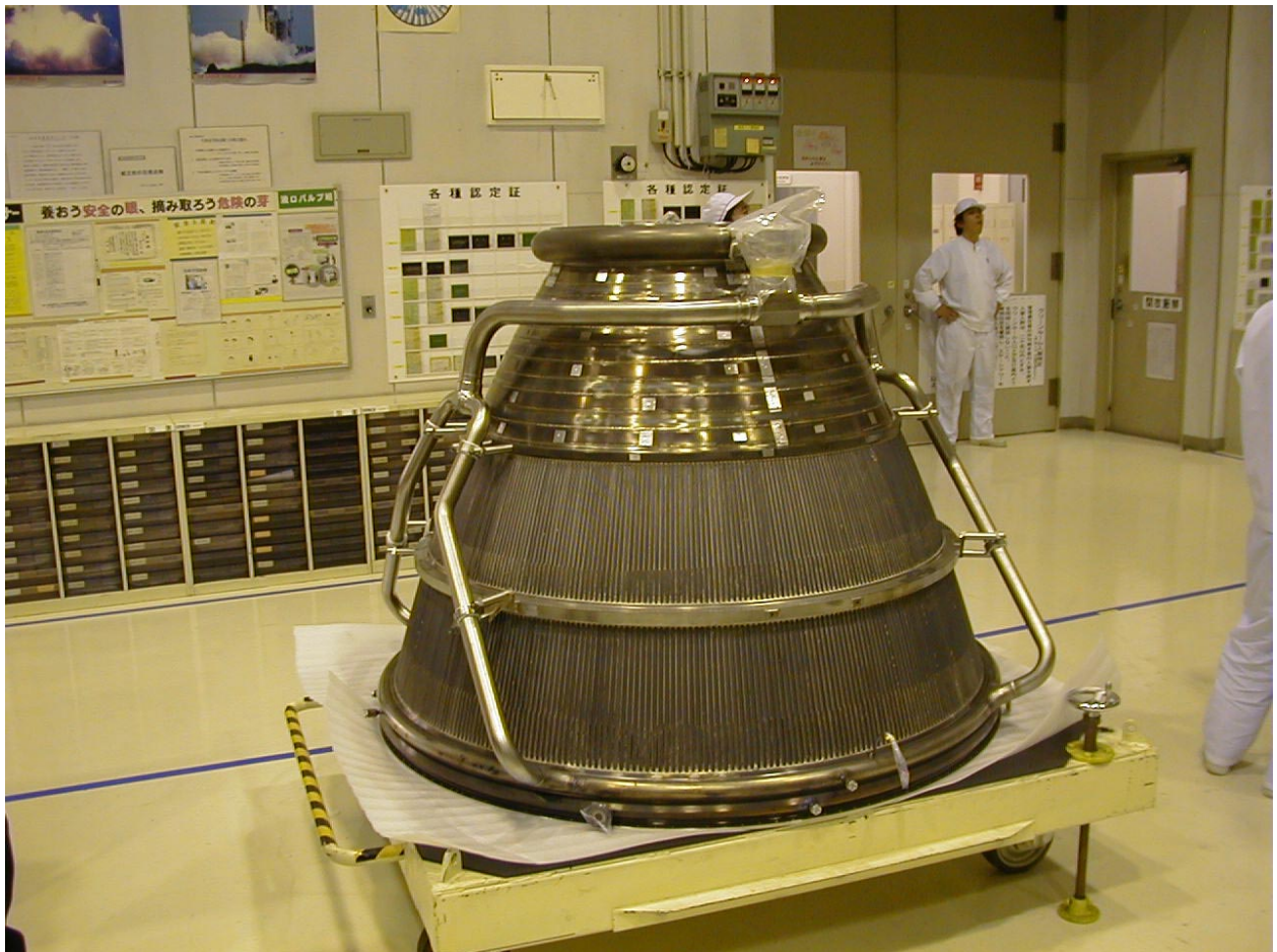
No. 8-1: The nozzle skirt of the LE-7A engine
