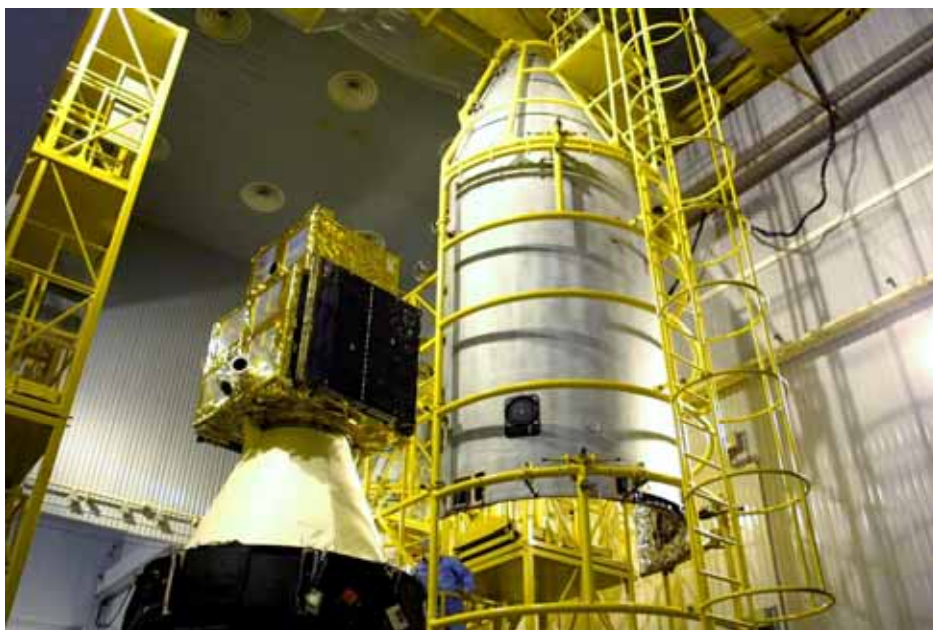
Fairing installation on SERVIS
