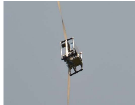
Fig.11 Team Okuzawa's climber which achieved the world record of 1,100m round trip in space elevator challenge 2013. (Photograph offered by JSEA/Akiyama) 19)
