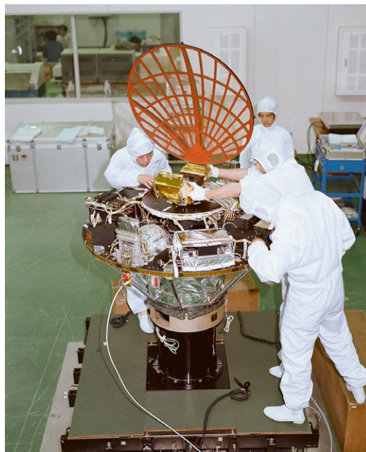
Snapshot of Integration Test for Installing Antenna to Explorer.
