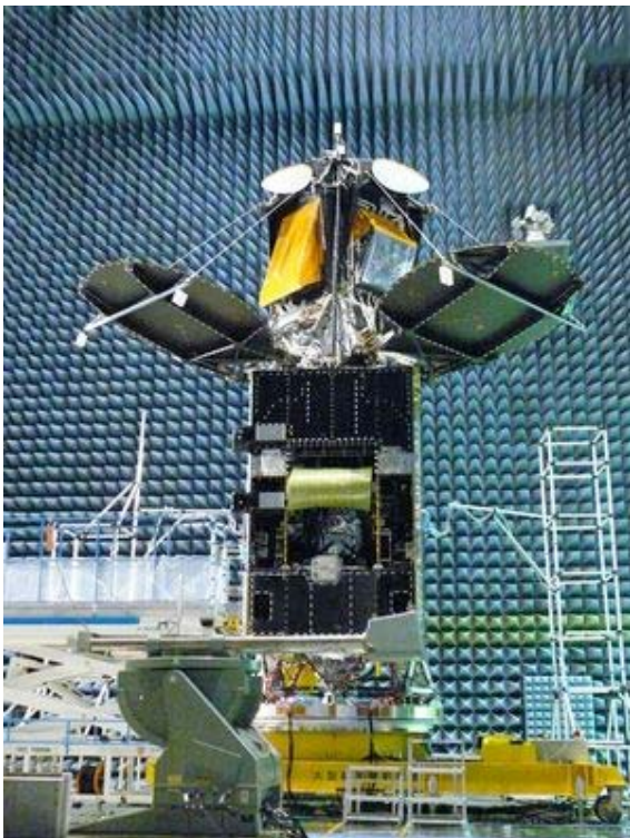
A state of a radio wave emission test
