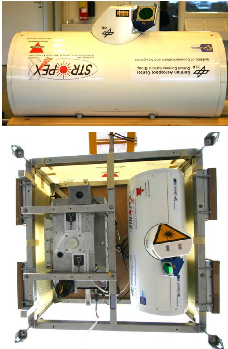
Fig. 4. Freespace Experimental Laser Terminal (upper) developed by DLR and the underneath view of the payload (lower) onboard the balloon [16]
