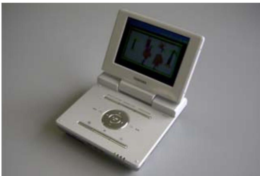
Figure.9 Mobile Receiving Terminal
