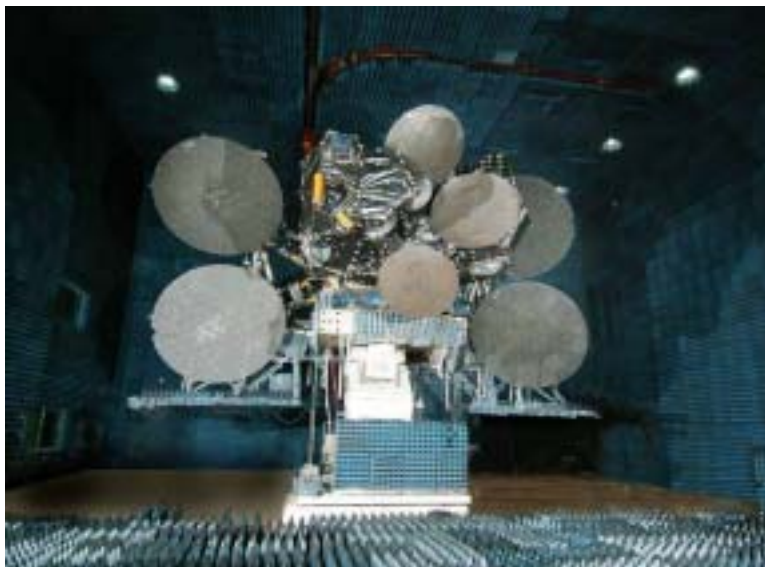
The IPSTAR satellite during CATR testing. (Courtesy of Space Systems/Loral & Shin Satellite Plc.)
