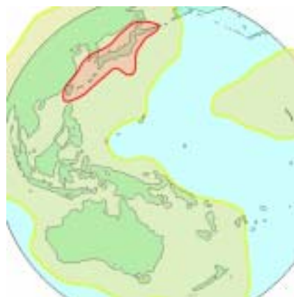
JCSAT-2A's Ku-band transponders (red) cover all of Japan, while its C-band transponders (yellow) cover Asia, Oceania and Hawaii.
