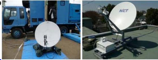
High data rate disaster communication between Matsushima Base and Iruma Base of JSDF using WINDS VSAT
