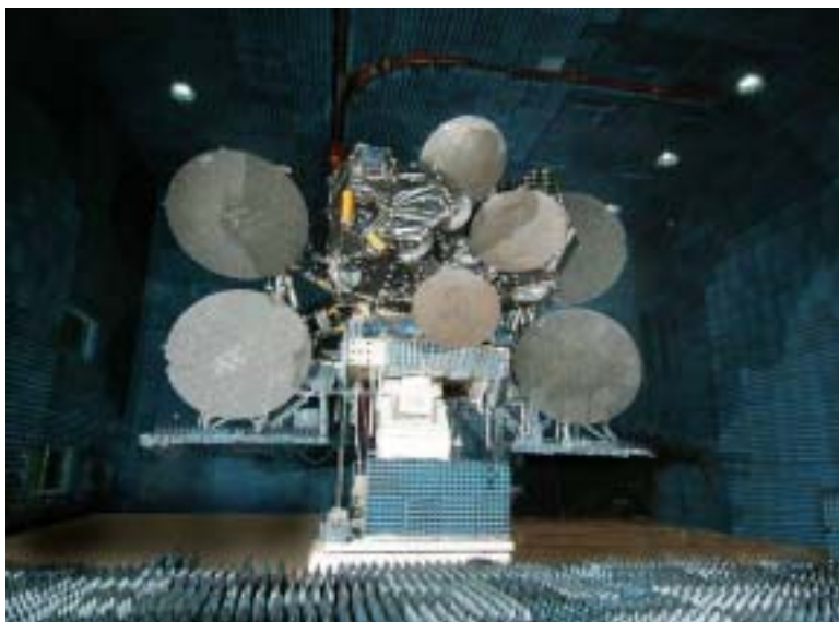
The IPSTAR satellite during CATR testing. (Space Systems/Loral & Shin Satellite Plc 提供.)
